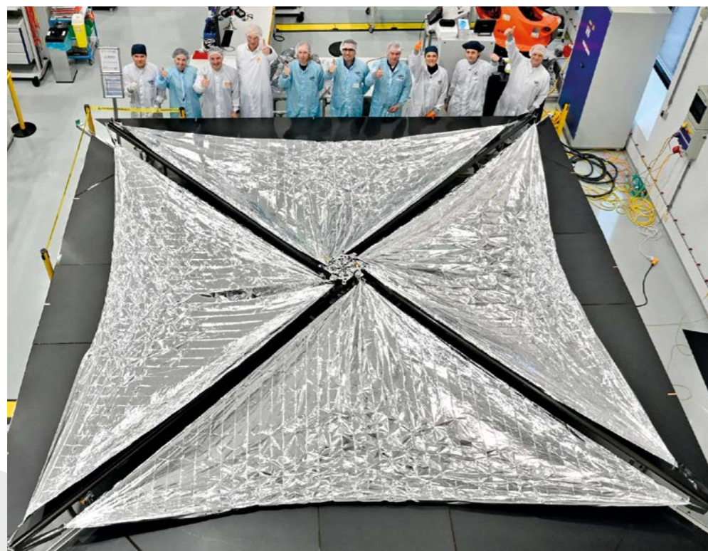
AEDO-L-Bremssegel erfolgreich im Labor entfaltet AEDO-L brake sails successfully deployed in the laboratory
